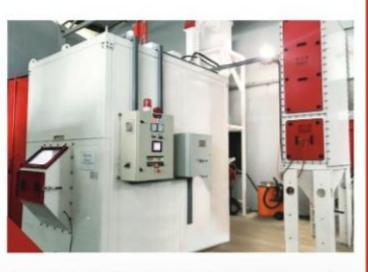
returned to the blasting pot. Precise abrasive metering permits micro adjustment to obtain the perfect abrasive flow rate. The blasting pressure is controllable from inside the blastroom, enabling the blasting operator to monitor and adjust the blasting parameters from inside the blastroom without having to stop blasting.
