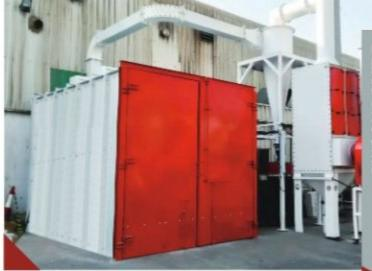
If the blastroom floor level is required to be flush with the surrounding factory floor level the entire blastroom can be situated into a pit approx. 275mm deep. During operation the abrasive is continually recovered and recycled, good reusable abrasive is separated from dust and oversize particles ensuring only correctly sized and fully cleaned abrasive is returned to the blasting pots.
